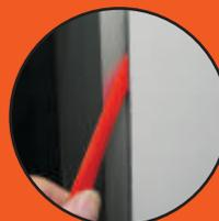
6. Move the object into position making light contact at one end. Once alignment looks correct, apply firm pressure at both ends and then pull the entrapped release liner at the 90° angle to expose the rest of the tape. Once liner fully removed, apply maximum pressure and clamp surfaces if practical to allow the bond strength to build.
