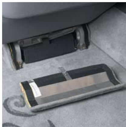
In and around seating, 3M Flame Resistant Scotchmate Reclosable Hook and Loop Fasteners secure a kickplate/access panel, hold seat cushions in place, and fasten carpeting to the floor.
